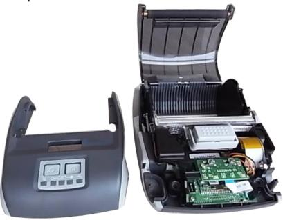
3. Use a tool to remove the shaft. Remove/Replace the media cover. (including the platen roller ass'y)
