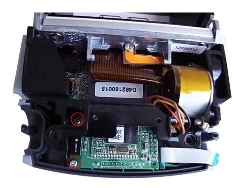
3. Disconnect the connector on the board.
