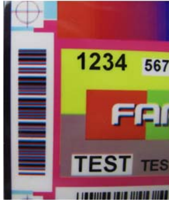
Black bar lines show horizontal mis-registration.
