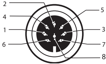
Figure 27: RS-232C Communications Port (8 pin Circular DIN)
